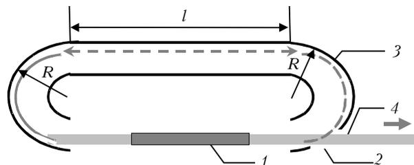
Fig. 2. Basic diagram of a simple ring cavity<sup>16</sup>: working medium 1; outlet 2; inner wall 3, along which a part of the laser beam is turned; laser beam 4.
