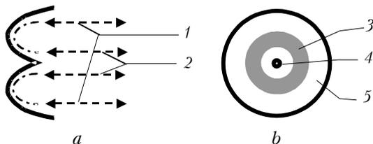
Fig. 4. Diagram of the grazing-incidence mirror of the X-ray cavity. Side (a) and end (b) views<sup>19</sup>: external 1 and internal 2 parts of the beam; absorbing ring 3; inner 4 and outer 5 working areas.
