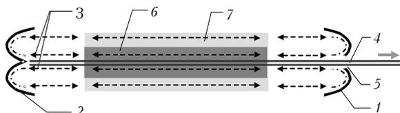
Fig. 5. Block-diagram of the ring cavity operating in the double-pass mode<sup>19</sup>: front mirror 1; back mirror 2; closed ray trajectories 3; laser beam 4; outlet 5; working medium 6 and 7 as the cavity operates in the single-pass and double-pass modes, respectively.
