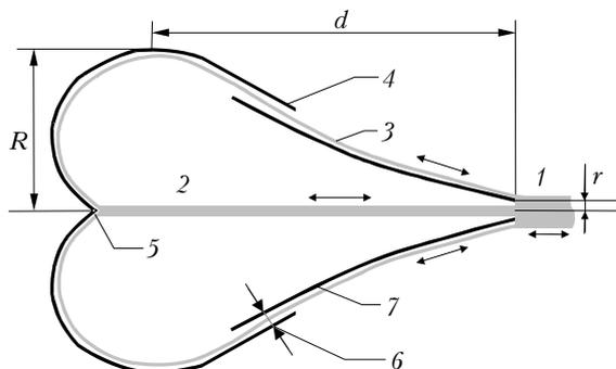
**Fig. 8.** Diagram of the pear-shaped reflector<sup>20</sup>: X-ray beam incident on the reflector inlet 1, inner 2 and outer 3 beams; large section of the reflector 4; cavity cone 5; cavity slit 6; external transportation mirror 7;  $R$  is the reflector radius;  $r$  is the radius of the reflector inlet;  $d$  is the part of the distance from inlet to the plane passing through the reflector cross section with the maximum area.
