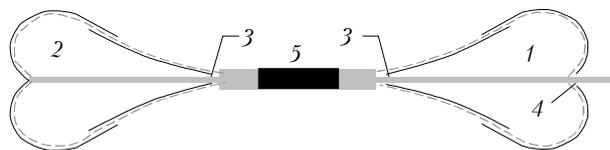
**Fig. 7.** Diagram of a cavity with pear-shaped reflectors.<sup>20</sup> Dashed curves show the trajectories of X-rays along the reflector surface: front and rear reflectors and their inlets 1, 2; inlets and outlet 3, 4; working medium 5.
