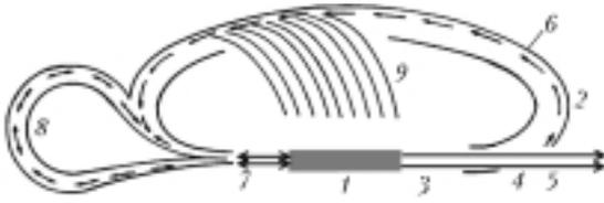
**Fig. 3.** Basic diagram of the ring cavity for X-ray laser<sup>17</sup>: laser working medium 1; ring cavity 2; beam from the face end of the working medium 3; outlet of the cavity 4; laser beam 5; beam turning in the cavity 6; part of the beam upon turning in the cavity and return ring 7; return ring 8; system of director surfaces 9.
