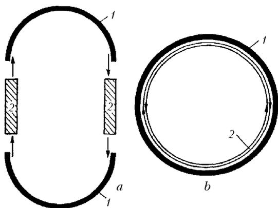
Fig. 1. Cavities with the circular-cylinder surfaces (1) and working medium of a laser (2): cavity with two mirror and working-medium sections (a) and single-section cavity with the counterpropagating pump beam (b) [Ref. 15].
