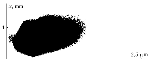
Fig. 4. Slit scan of the natural glow of the plasma jet generated by the short-pulse laser radiation.
