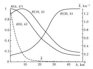
Fig 1b. Correlation between absorption coefficients at different heights.
