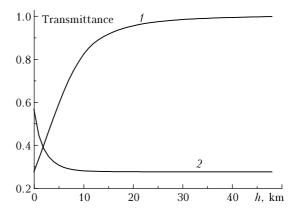
**Fig. 1c.** Calculation of atmospheric transmittance by the line-by-line method. Vertical paths: fixed upper boundary  $h_{\rm up} = 50$  km, variable lower boundary (1); fixed lower boundary  $h_{\rm low} = 0$  km, variable upper boundary (2). Spectral range of 740–760 cm<sup>-1</sup>.
