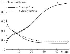
**Fig. 2c.** Calculation of atmospheric transmittance by the line-by-line method (solid curve) and by the *k*-distribution method (dashed curve). Designations are the same as in Fig. 1c. Spectral range of 1027-1032 cm<sup>-1</sup>.
