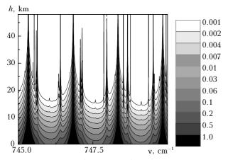
Fig. 1a. Height and spectral dependence of the  $CO_2$  molecular absorption coefficient, in  $km^{-1}$  (fragment of the spectrum).
