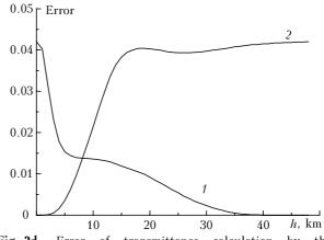
**Fig. 2d.** Error of transmittance calculation by the k-distribution method. Designations are the same as in Fig. 1c.
