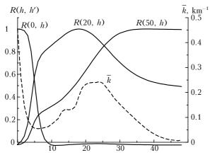
Fig. 2b. Correlation between absorption coefficients at different heights.
