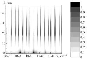
Fig. 2a. Height and spectral dependence of the molecular absorption coefficient in the gas mixture of  $H_2O$ ,  $CO_2$ , and  $O_3$ , in km<sup>-1</sup>.
