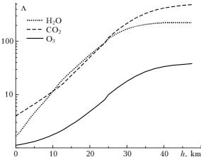
Fig. 3. Height dependence of the lacunarity parameter for different absorbing gases in the spectral range of 1027-1032 cm<sup>-1</sup>.
