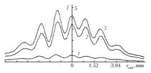
Fig. 3. Interferograms for solar aureole in the Earth's atmosphere at the input aperture of 1.62 mm in diameter; the distant aureole (1); at the intermediate position of the interferometer axis (2); the near aureole (3). The scale value of the vertical axis is 0.05 V/div.
