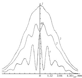
**Fig. 2.** Interferograms when aiming the interferometer axis at the solar center. For curves 1, 2, and 3 the entrance apertures had diameters of 0.25, 1.62, and 3.0 mm, respectively. The scale values of the vertical axis for curves 1, 2, and 3 are equal to 0.25, 1, and 2.13 V/div.
