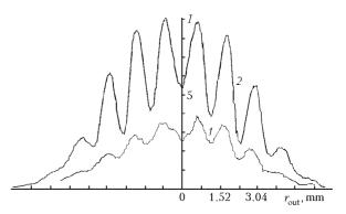
Fig. 4. Interferograms for solar aureole in the Earth's atmosphere at the entrance aperture of 3.0 mm: the distant aureole (1); the near aureole (2). The scale value of vertical axis is 0.05 V/div.
