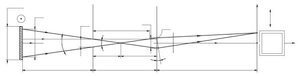
Fig. 1. Optical arrangement of the interferometer.
