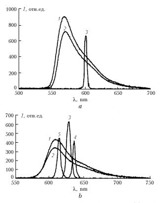
**Fig. 3.** Emission spectra of Rhodamine 6G (a) and phenalemine-512 (b) in ethanol (1-4) and PMMA (5): laser-induced fluorescence (1), TPLu (2), lasing (3-5).
