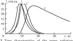
Fig. 5. Time characteristics of the pump radiation (1), TPLu (2), and TPL (3) of phenalemine 512, and spark (4).
