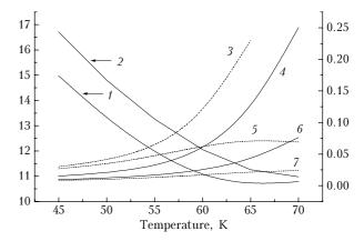
Fig. 4. Temperature dependence of optimal  $\lambda_c$  and minimal NETD for single-layer and many-layer HIP-detectors.
