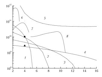
**Fig. 2.** Wavelength dependence of detectability for varioustype photoemissive detectors.
