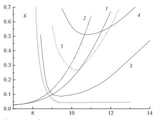
Fig. 3. Dependence of the noise equivalent temperature difference on  $\lambda_c$  for HIP detectors under different radiation recording conditions.
