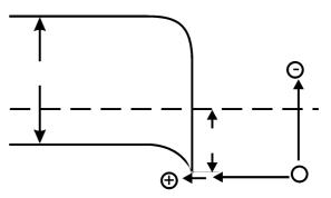
Fig. 1. Energy band diagram of PtSi/p-Si Schottky-barrier detector with internal photoemission.
