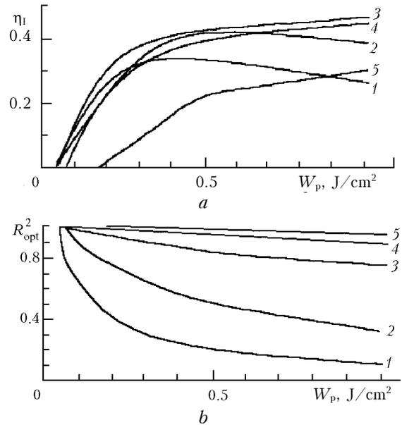
**Fig. 3.** The conversion coefficient (a) and the optimal reflection coefficient of the exit mirror (b) for OPO based on  $\text{AgGaSe}_2$  pumped by radiation at  $\lambda_p = 2.1$   $\mu\text{m}$  vs. the pump energy density at different values of  $\gamma$ :  $10^{-3}$  (1),  $10^{-4}$  (2),  $10^{-5}$  (3),  $10^{-6}$  (4), and  $10^{-7}$  (5).
