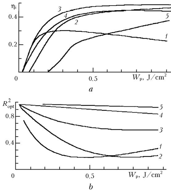
**Fig. 2.** The conversion coefficient (a) and the optimal reflection coefficient of the exit mirror (b) for OPO based on  $\text{HgGa}_2\text{S}_4$  pumped by radiation at  $\lambda_p = 2.1$   $\mu\text{m}$  vs. the pump energy density at different values of  $\gamma$ :  $10^{-3}$  (1),  $10^{-4}$  (2),  $10^{-5}$  (3),  $10^{-6}$  (4), and  $10^{-7}$  (5).
