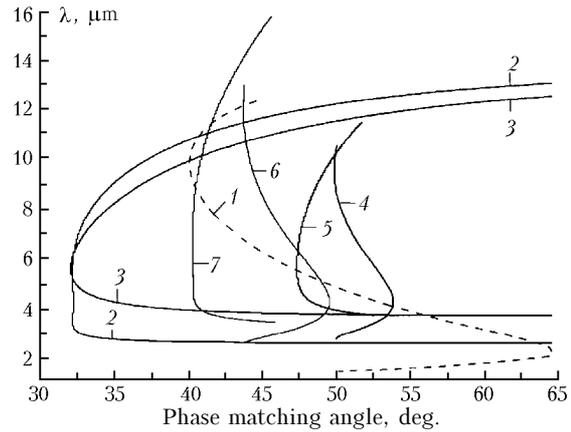
**Fig. 1.** Conversion phase matching curves for OPO in HgGa<sub>2</sub>S<sub>4</sub> crystal pumped by 1.06  $\mu$ m (1), 2.1  $\mu$ m (2), and 2.8  $\mu$ m (3) radiation; ZnGeP<sub>2</sub> crystal pumped by 2.1  $\mu$ m (4) and 2.8  $\mu$ m (5) radiation; and AgGaSe<sub>2</sub> crystal pumped by 2.1  $\mu$ m (6) and 2.8  $\mu$ m (7) radiation.
