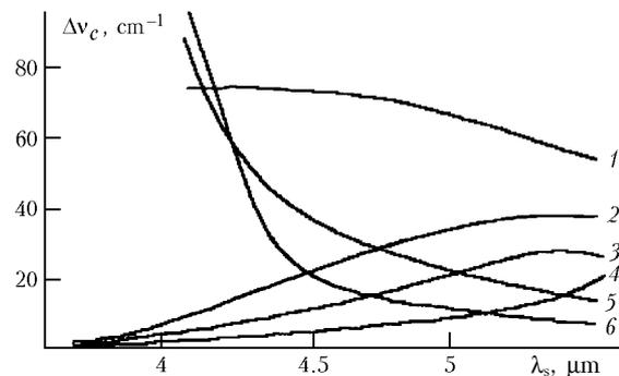
Fig. 5. Gain band of OPO based on ZnGeP<sub>2</sub> [ $\lambda = 2.1 \mu\text{m}$  (1),  $\lambda = 2.8 \mu\text{m}$  (4)]; AgGaSe<sub>2</sub> [ $\lambda = 2.1 \mu\text{m}$  (6),  $\lambda = 2.8 \mu\text{m}$  (2)]; HgGa<sub>2</sub>S<sub>4</sub> [ $\lambda = 1.06 \mu\text{m}$  (5),  $\lambda = 2.1 \mu\text{m}$  (3)].
