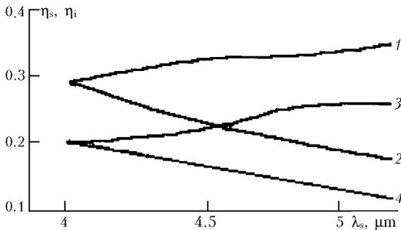
Fig. 4. Coefficient of conversion in AgGaSe<sub>2</sub> [ $\lambda_s$  (1),  $\lambda_i$  (2)] and ZnGeP<sub>2</sub> crystals [ $\lambda_s$  (3),  $\lambda_i$  (4)] for  $\gamma = 10^{-4}$ ,  $R^2 = 0.65$ ,  $W_p = 0.5 \text{ J/cm}^2$ ,  $\lambda_p = 2.1 \mu\text{m}$ .
