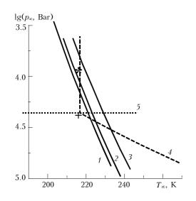
The difference between the crystallization  $T_i$  and condensation  $T_c$  temperatures is negligible. Mass concentration of crystal aerosol  $Y_i$  at  $S_{\infty} = 0$ , near the low and upper thresholds of condensation (T = 222.25 K;  $p_{\infty c} \approx 0.259$  Bar,  $h \approx 10$  km and  $T_{\infty} = 216.7$  j;  $p_{\infty c} \approx 0.147$  Bar,  $h \approx 14$  km), is  $1.27 \cdot 10^{-4}$ and  $1.32 \cdot 10^{-4}$ , respectively; the water ice content
