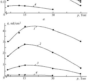
Fig. 7. Output energy (a) and output energy density (b) of nitrogen laser vs. nitrogen pressure in discharge tubes of different diameter d = 2.2 (1), 3.4 (2), 6.8 (3), and 9.5 mm (4) (tube length of 200 mm,  $C_2 = 330 \text{ pF}$ ).
