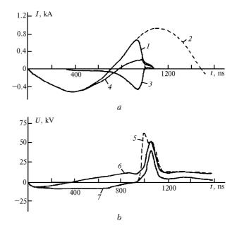
**Fig. 4.** Oscillograms of current and voltage at idle operation of the setup ( $C_1 = 16.5$  nF,  $C_2 = 0$ ):  $I_2$  (1),  $I_2$  at the short-circuit opening switch (2),  $I_3$  (3),  $I_4$  (4),  $U_1$  (5),  $U_3$  (6), and  $U_2$  (7).
