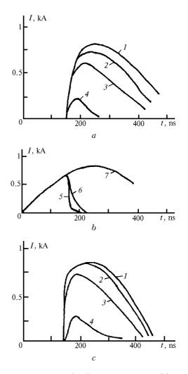
**Fig. 2.** Experimental (a, b) and calculated (c) current oscillograms at  $C_2 = 0$ ;  $I_1(a, c)$  at  $R_L = 0$  (1), 5 (2), 20 (3), and 200  $\Omega$  (4);  $I_2$  (b) at  $R_L = 0$  (5) and 200  $\Omega$  (6) and at short-circuit switch (7).
