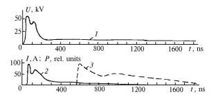
**Fig. 10.** Oscillograms of voltage across gas-discharge gap (1), discharge current (2), and CO<sub>2</sub> laser pulse (3) (CO<sub>2</sub>:N<sub>2</sub>:He =1:3:3,  $C_1$  = 16.5 nF, tube length is 400 mm, d = 9.5 mm, p = 27 Torr).
