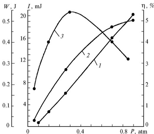
**Fig. 1.** Energy dissipated in a gas (1), emitted energy (2), and efficiency (3) as functions of the active medium pressure  $\text{SF}_6:\text{H}_2 = 7:1$ .
