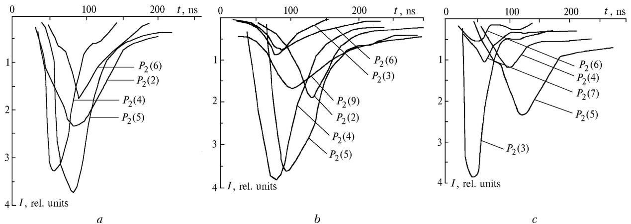
**Fig. 5.** Time behavior of intensity of separate lines of the  $P_2$  transition in the mixture  $\text{SF}_6:\text{H}_2 = 7:1$  at different pressure: 0.82 (a), 0.344 (b), and 0.096 atm (c).
