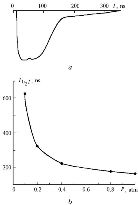
**Fig. 4.** Oscilloscope of radiation pulse (a) ( $p = 0.344$  atm) and pressure dependence of the pulse duration at halfmaximum (b) in the mixture  $\text{SF}_6:\text{H}_2 = 7:1$ .
