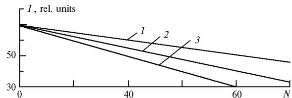
**Fig. 3.** Relative change of the radiation energy vs. number of accelerator turns-on in the presence of an absorber of 4 (1), 6 (2), and 0  $\text{cm}^3$  (3) in volume.
