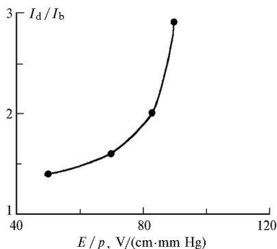
**Fig. 2.** Output laser energy as a function of  $E/p$ .  $I_b$  and  $I_d$  are the radiation energy in the case of active medium excitation by  $e$ -beam and by an  $e$ -beam-initiated discharge, respectively. Mixture  $\text{SF}_6:\text{H}_2 = 7:1$ ,  $p = 0.184$  atm.
