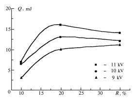
**Fig. 2.** Radiation power for the mixture (Ne) Xe:HCl = 5:1 (4 Torr) at the pressure of 3.5 atm vs. the reflectance of the output mirror and the charging voltage.
