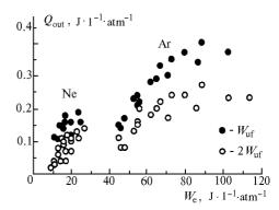
Fig. 4. Specific output power  $Q_{\rm out}$  vs. the specific energy contribution  $W_{\rm e}$  and the preionizer intensity in argon and neon mixtures.
