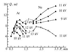
Fig. 3. Typical dependence of the output power emitted from the mixture Xe:HCl = 5:1 (4 Torr) with buffer gases on the working pressure, charging voltage, and the preionization intensity.
