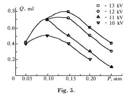
Besides, we have studied with this laser the output parameters of a N<sub>2</sub> laser. Figure 5 shows the typical dependence of the nitrogen laser output power on the working pressure and charging voltage. The maximum power of 0.8 mJ was observed at the pressure of 0.15 atm and  $U_0 = 13$  kV. The pulse length at halfmaximum was 5 ns. It should be noted that this pump system provides for high output parameters of
