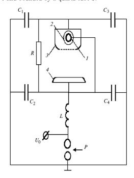
**Fig. 1.** Electric circuitry of the EKSIK-2 laser: recharge inductance L and triggered switch P.
