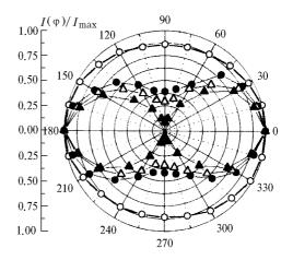
**Fig. 2.** Angular diagram of polarization degree of radiation reflected from the asphalt cover surface under different conditions of the surface: dry asphalt cover ( $\circ$ ); snow ( $\bullet$ ); wet asphalt cover ( $\Delta$ ); the ice cover ( $\sigma$ ).
