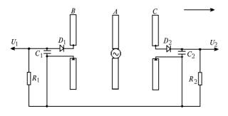
**Fig. 3.** Block-diagram of the recording technique of the dielectric constant variation at the line separating two media. A is the transmitting antenna, B and C denote the receiving antennas.
