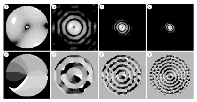
FIG. 1. Real-zeros and the phase vortices of a wave and its Fourier transforms when propagating through an inhomogeneous medium ( $C_n^2 = 10^{-14} \text{ m}^{-2/3}$ , L = 2000 m). Intensity of the wave with the real zero at the center of the Hartmann subaperture (+) (1) and the corresponding phase (2). Focal spots (3, 5, and 7) and the phase (4, 6, and 8), which correspond to the focal spots, located opposite to the wave with the real zero (1 and 2) when increasing the size of the subaperture.
