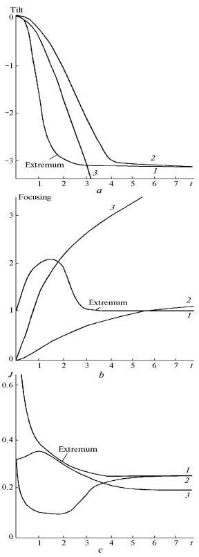
FIG. 2. Changes of the extremum coordinates (tilt (a) and defocusing (b)) and the criterion J(t) (c) at heating of a medium by a beam (curve 1 in all the figures) and corresponding changes in those due to control (curve 2 corresponds to  $\alpha_{Tilt} = 2.5$ ,  $\alpha_{Foc} = 0.2$ , curve 3 to  $\alpha_{Tilt} = 2.5$ ,  $\alpha_{Foc} = 0.5$ ).
