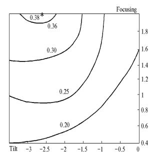
FIG. 3. Distribution of J(t) for a frozen thermal lens.
