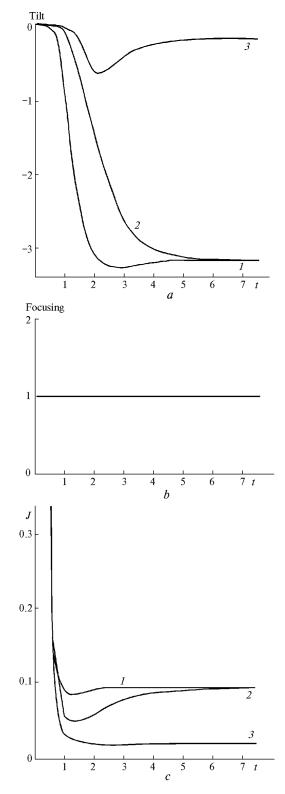
FIG. 6. Control over tilt,  $\alpha_{Tilt} = 10$  (curve 1) and  $\alpha_{Tilt} = 5$  (curve 2), termination of the control in vicinity of the global maximum;  $\alpha_{Tilt} = 2.5$  (curve 3), termination of the control in a local maximum.
