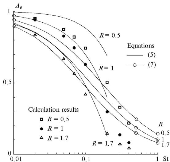
FIG. 4. Calculation results for the efficiency of outer aspiration.
