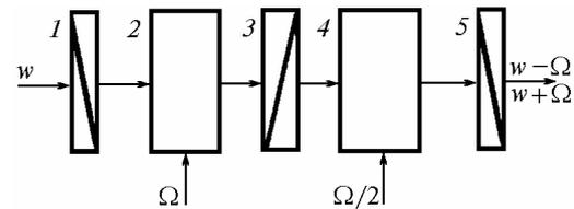
FIG. 2. Structure scheme of the two-modulator electrooptical device for transformation of single-frequency coherent radiation into bi-frequency one: polarizers (1, 3, and 5); electrooptical modulators (2 and 4).
