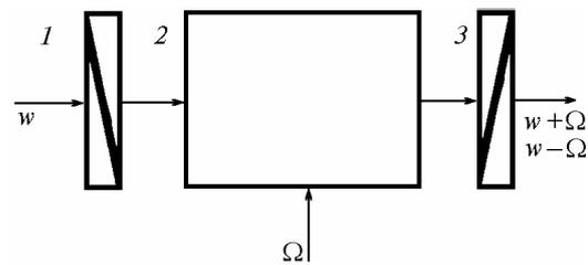
FIG. 1. Structure scheme of the single-modulator electrooptical device for transformation of single-frequency radiation into bi-frequency one: polarizers (1 and 3) and electrooptical modulator (2).
