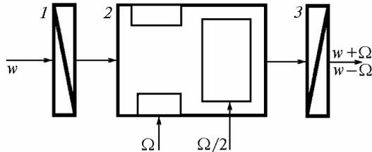
FIG. 3. Structure scheme of the single-crystal electrooptical device for transformation of single-frequency coherent radiation into bi-frequency one: polarizers (1 and 3); electrooptical crystal with two pairs of control electrodes (2).
