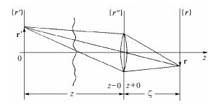
FIG. 1. Model of the image transfer through the turbulent atmosphere:  $\mathbf{r}'$  is the point source coordinate in the object plane  $\{\mathbf{r}'\}$ ;  $\mathbf{r}''$  is the coordinate in the lens plane;  $\mathbf{r}$  is the coordinate in the image plane; z is the distance between the object plane  $\{\mathbf{r}'\}$  and a lens;  $\zeta$  is the distance between the image plane  $\{\mathbf{r}\}$  and a lens;  $\zeta \approx f$  at  $f \ll z$ , where f is the focal length of a lens.
