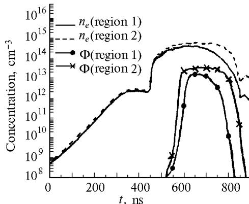
FIG. 4. Electron concentrations  $n_{ei}(t)$  and photon concentrations  $F_i(t)$  for the discharge regions  $i = 1, 2$ .
