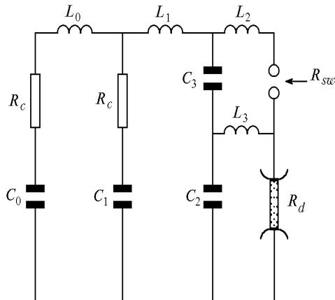
FIG. 1. Block-diagram of the equivalent circuitry.
