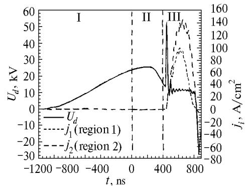
FIG. 2. Time behavior of the plasma voltage  $U_d$  and current density  $j_i$  in some regions  $i$  of the discharge: recharge stage (I), low-current stage (II), high-current stage (III).
