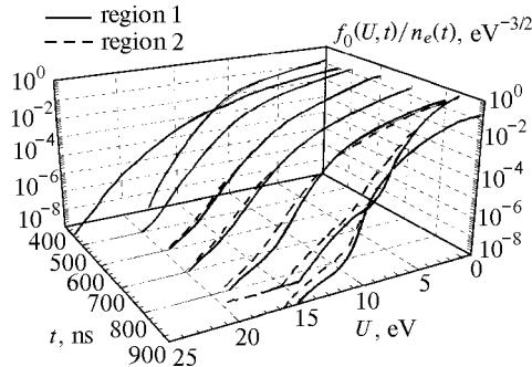
FIG. 3. Time behavior of the isotropic part of the electron velocity-distribution function.
