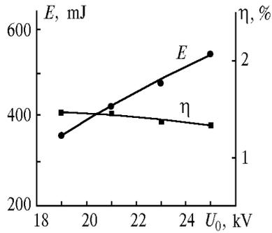
FIG. 3. Energy of ArF-laser generation  $E$  and lasing efficiency  $\eta$  as functions of the charging voltage  $U_0$  in the mixture He:Ar:F<sub>2</sub> in ratios 79.7:20:0.3.
