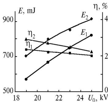
FIG. 4. Energy of KrF-laser generation and lasing efficiency as functions of the charging voltage  $U_0$  in mixture He:Kr:F<sub>2</sub> in ratios 89.8:10:0.2 ( $e_1$ ,  $\eta_1$ ) and He:Ne:Kr:F<sub>2</sub> in ratios 49.9:49.9:10:0.2 ( $e_2$ ,  $\eta_2$ ).
