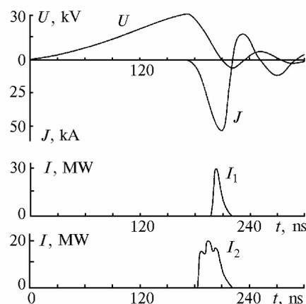
FIG. 2. Waveforms of pulses of the voltage on the discharge gap  $U$ , discharge current  $J$ , and laser generation  $I_1$  (ArF) and  $I_2$  (KrF) for  $U_0 = 19 \text{ kV}$ .
