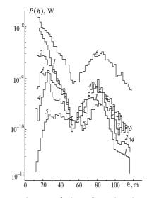
FIG. 4. Distribution of the reflected radiation power over the multiple scattering orders. Numbers of the curves 1-5 correspond to the order of multiple scattering and 6 is the total signal power P(h).
