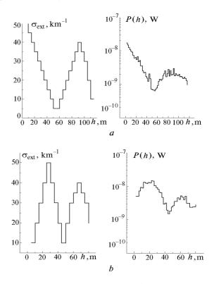
FIG. 3. The return signal power P(h) for the shape of  $\sigma_{ext}(h)$  profile with several maxima.
