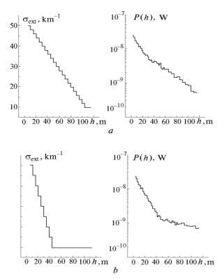
FIG. 1. Lidar return P(h) as a function of the extinction coefficient profile  $\sigma_{ext}(h)$ .
