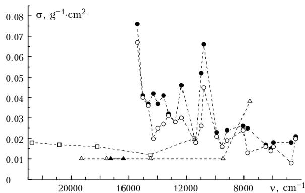
FIG. 2. The atmospheric air absorption cross-sections from Ref. 1 (●), from Ref. 1 with the account for selective absorption (○), from Ref. 2 (□), and the data presented by the authors (Δ).
