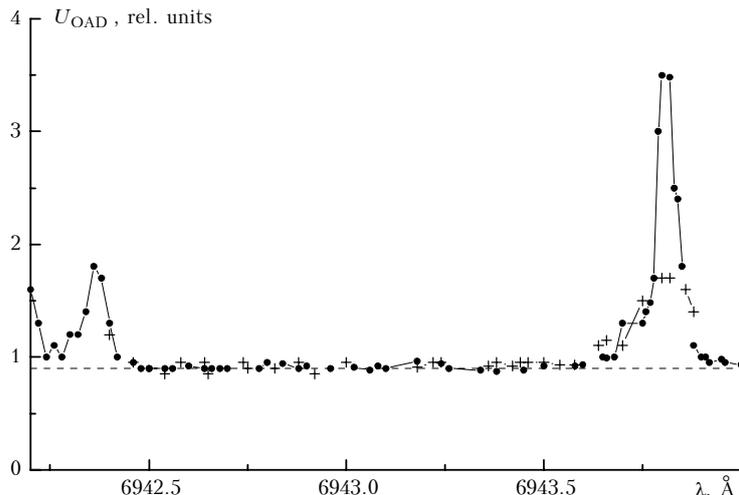
FIG. 1. Absorption spectrum of atmospheric air in the range of the ruby laser temperature tuning.  $P = 300$  mm Hg, (●) correspond to  $N_{H_2O} = 5.5$  g/m<sup>3</sup> and (+) to dried air; the background level is denoted by the dashed curve.
