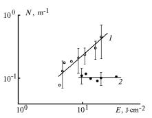
FIG. 2. Dependence of the linear concentration of optical break down cells on the laser radiation energy density: (1) 15 min fog lifetime on the measurement path, (2) 30 min and longer lifetime.
