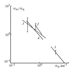
FIG. 3. Influence of the atmospheric optical and meteorological state on the nonlinear extinction coefficient for  $CO_2$  laser radiation: (1) fog, (2) drizzle, (3) rain, and (4) snow.
