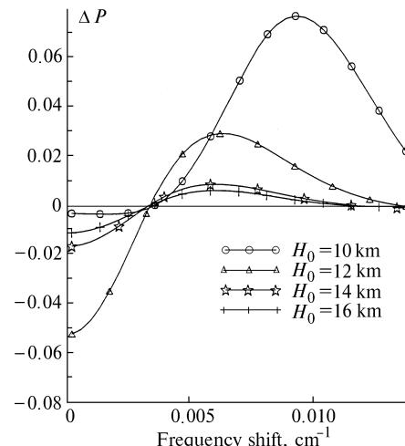
FIG. 2. Spectral dependences of the differences between the monochromatic transmission functions for the Voigt and Galatry lineshapes of the  $\text{H}_2\text{O}$  line at different sighting heights ( $v_0 = 3950.271 \text{ cm}^{-1}$ ).
