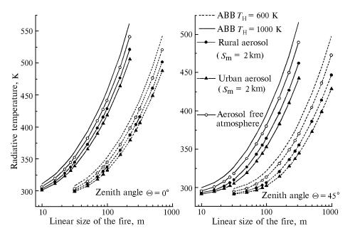
FIG. 1. Radiative temperature as a function of linear size of the fire.
