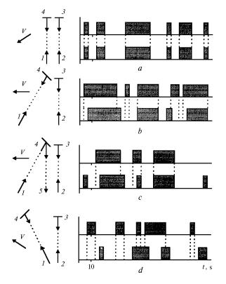
FIG. 2. Correlation of the fluctuation processes on the horizontal paths. To the left is set out the geometry of the basic and auxiliary double passage paths, to the right are shown durations of the stochastic beam state I (dashed rectangles) and quasiregular state II. Section 2-3 corresponds to the basic path, 1-4 to the auxiliary path. The upper set of the temporal intervals refers to the basic path, the lower set to the auxiliary path.
