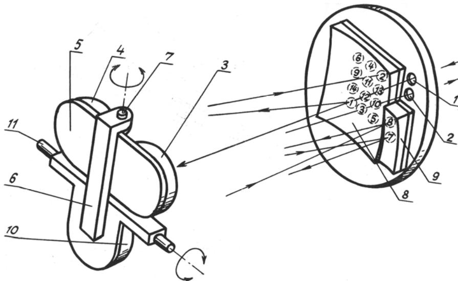
Fig. 1. Three-objective multipass matrix-array system
