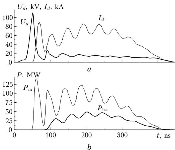
**Fig. 4.** Calculated time dependence of the pump power and the output laser power (b), voltage across the discharge gap and discharge current (a) for the mixture Ne : Xe : HCl = 2500 : 20 : 2.5;  $p = 3.5$  atm at pumping from the generator with the inductive storage.
