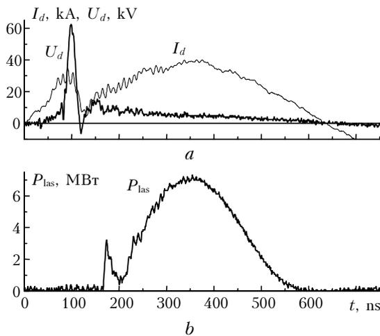
**Fig. 3.** Characteristic oscillograms of voltage across the laser gap, discharge current of the primary storage  $C_0 = 550$  nF (a) and lasing (b) of the XeCl laser with the inductive storage, an active volume of  $100 \times 4 \times 2$  cm; mixture Ne:Xe:HCl = 3 atm:10:1 Torr;  $U_0 = 20$  kV.
