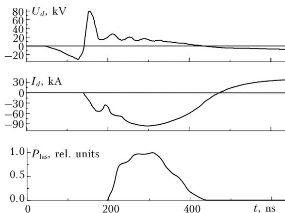
**Fig. 2.** Characteristic oscillograms of the voltage across the laser gap, discharge current, and lasing in the mixture Ne : Xe : HCl = 2100 : 10 : 1 at a pressure of 4 atm. The charging voltage of the capacitor  $C_{pr}$  is equal to 50 kV.
