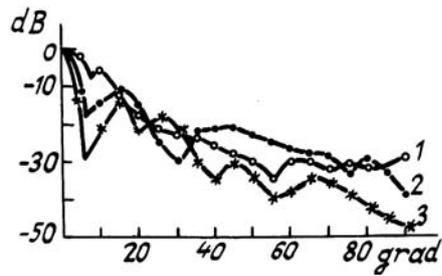
FIG. 2. Directional pattern of a selective acoustic antenna: 1) directional pattern of the horn; 2) directional pattern of an antenna with phase reversal in the even Fresnel zones; 3) same, but with phase reversal in the odd Fresnel zones.
