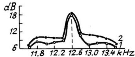
FIG. 1. The amplitude-frequency characteristics of the phase zone plates: 1) with phase reversal in the odd Fresnel zones and 2) with phase reversal in the even Fresnel zones.
