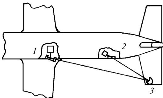
Fig. 1. Layout of instrumentation placed on board the aircraft.
