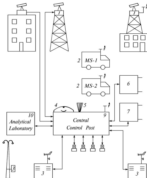
FIG. 2. Configuration of the system of monitoring of the atmospheric air.
